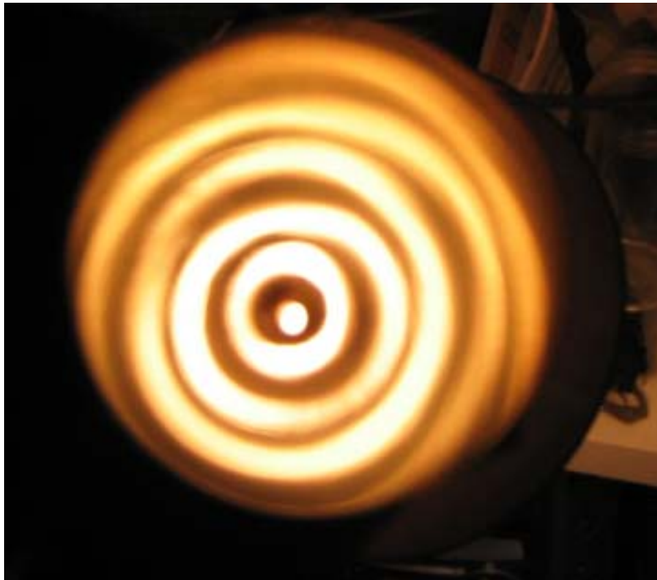
Pinhole diffraction—Rings produced by larger diameter source#1
