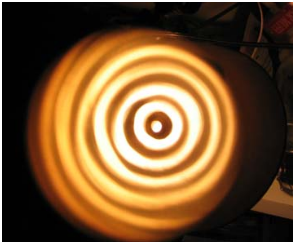
Pinhole diffraction—Rings produced by larger diameter source#2
